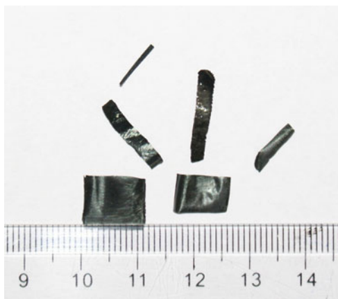
Fig. 7 Photograph of free-standing conducting PTT films prepared from BFEE at the constant applied potential of 0.80 \text{ V vs. Ag/AgCl}
